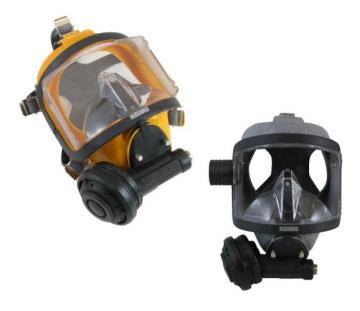
The **Divator breathing valve** is one of the best-tested breathing valves available. It will perform even in the most extreme conditions: mud, oil and fast flowing cold currents does not have a serious impact on the performance. The breathing valve is balanced and maintained extremely low breathing resistance at all diving depths even if variations occur in the secondary pressure.
